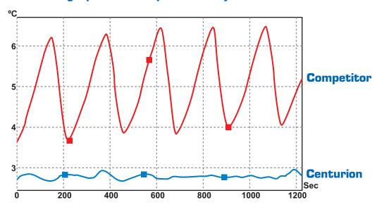
Centurion has a set temperature of 3°C, and our competitor of 4°C. This allows us to separate the target areas, to show how each machine regulates the temperature. Both refrigeration units use the same air probes, temperature units, and have the probes set at the same distance from the rotor, and finally, the correct vertical distance to the optimum the tube area.
